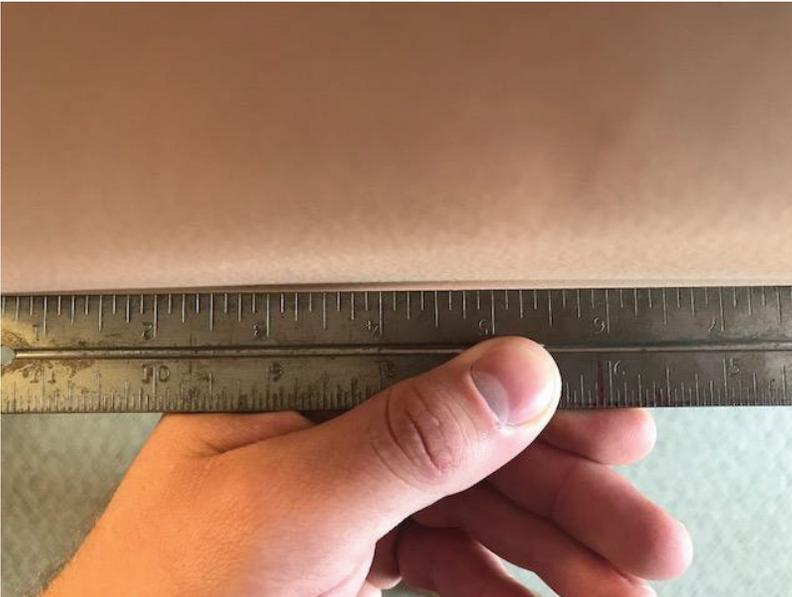
Photo 2: Photo of straight edge used to evaluate wall flatness for Glass Units.
