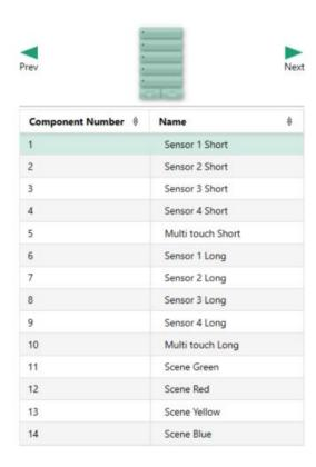
The numbers of the sensors corresponds with the following physical buttons on the Sentido/Fibonacci keypad electronics, when installed correctly/upright:
